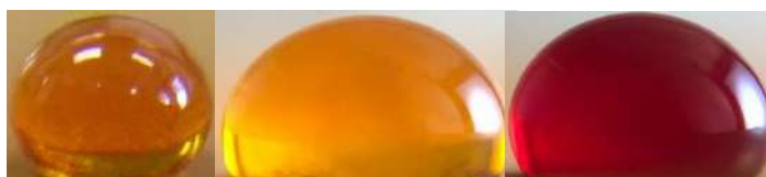
Figure 6. Titration experiments showing the color change of PR indicator depending on the pH value. The color of PR droplet before mixing (left), the color of PR droplet mixed with an acid droplet (middle) and the color of PR droplet when mixing with a base droplet.
