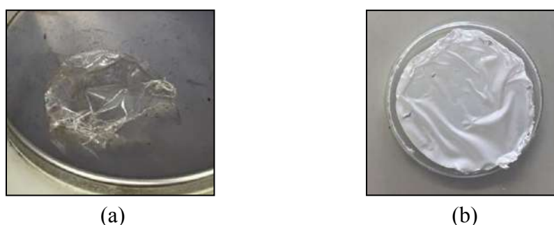
Figure 2. physical appearance of films (a) pure gelatin film (b) gelatin/nano-TiO 2 blended films
